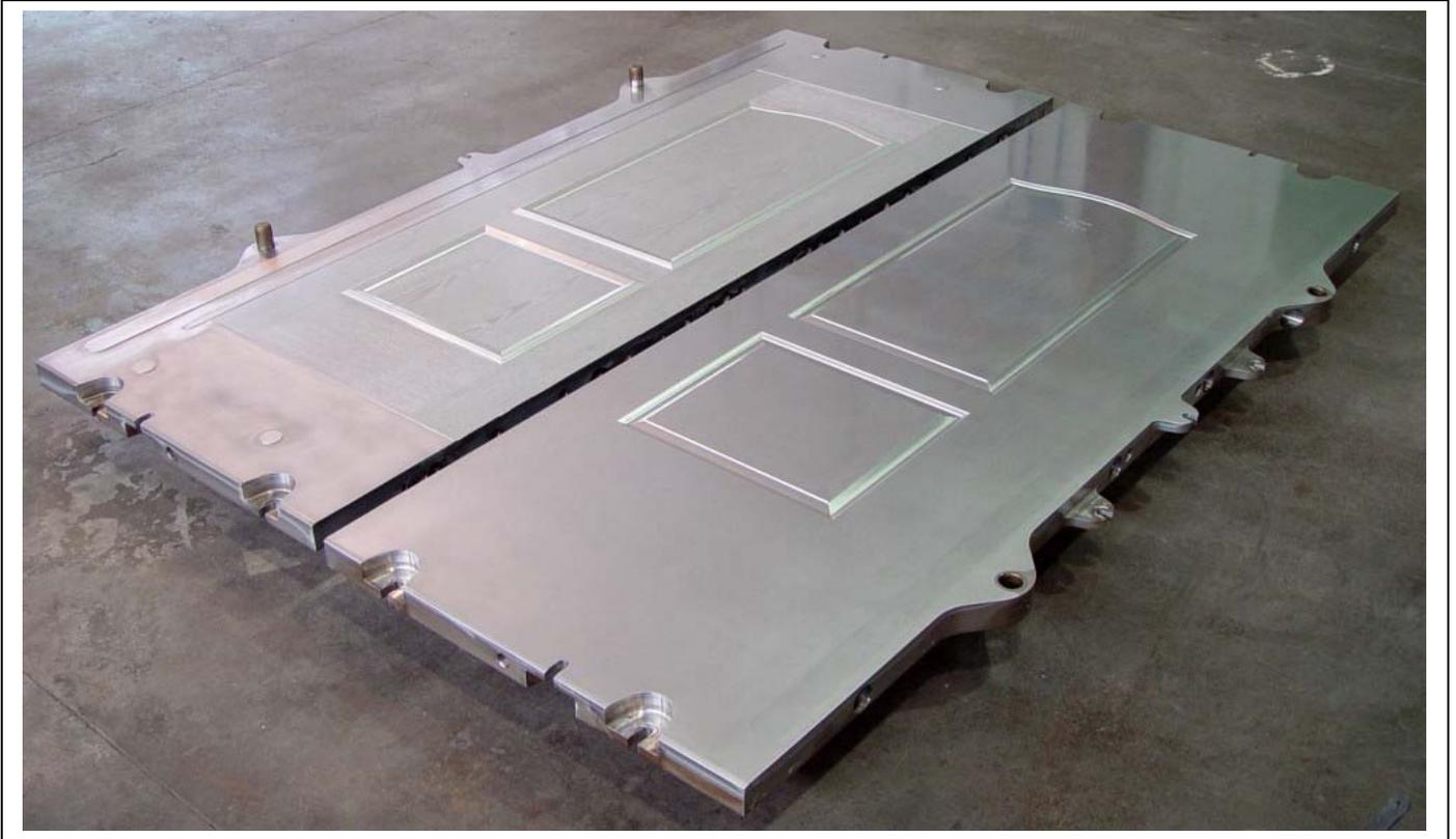
• *Core and cavity set of doorskin mold*
